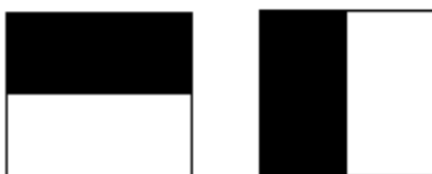
Fig. 4. Haar-wavelet response in x and y direction
